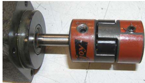
Flexible coupling on pump shaft
