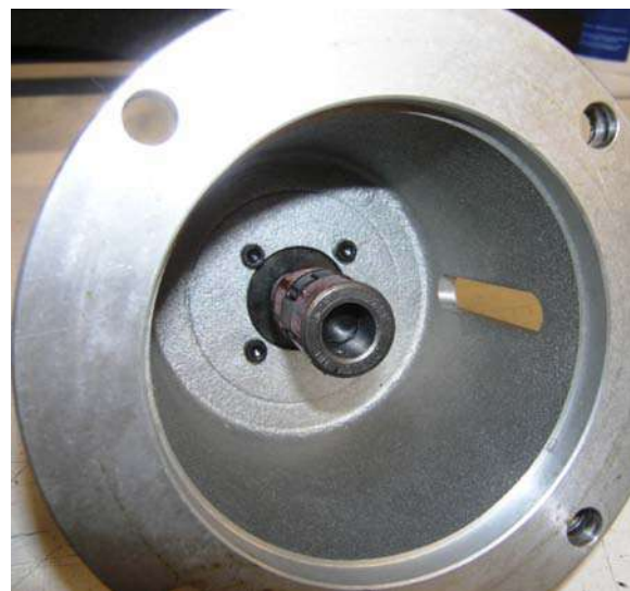
Flexible coupling with 56C bell housing
